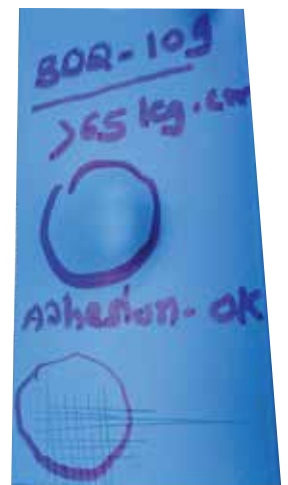
Aakar maintains batch record of scratch & impact tests on powder coated panels
