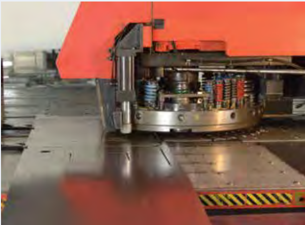
CNC Turret Punch ensures accuracy
