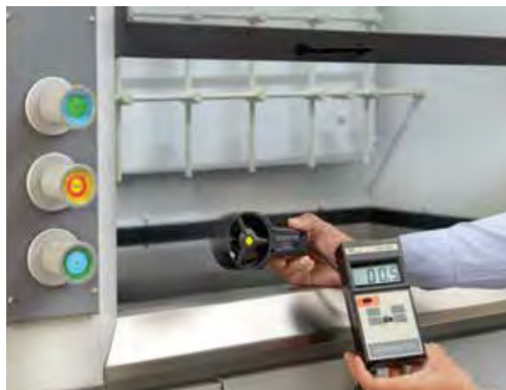
Required average face velocity 0.5 m/s
